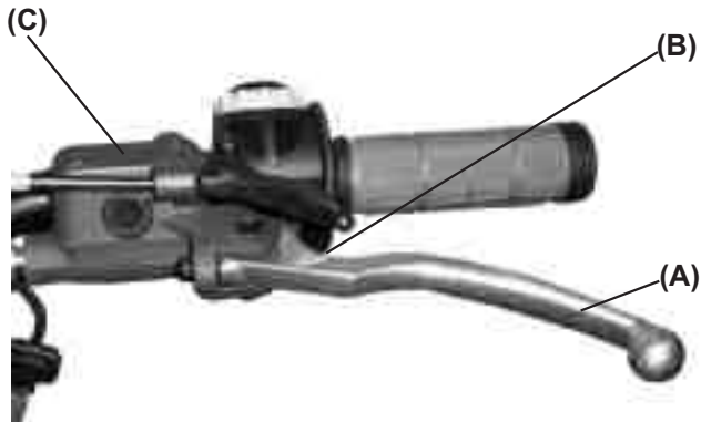
(A). Clutch Lever. (B). Clutch cylinder piston rod. (C). Hydraulic fluid tank.
