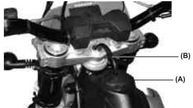
(A). Fuel cap. (B). Fuel vent hose.
